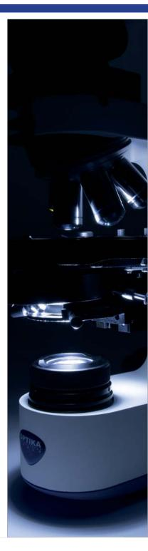
Low position focus and stage controls allow a fast and comfortable operation. Frequently used controls as light intensity adjustment and diaphragm are also placed in the lower part of the stand and enable operation without having to take the eyes off the specimen. All optical heads are equipped with high-point eyepieces and dioptric adjustment, for the best viewing experience.
